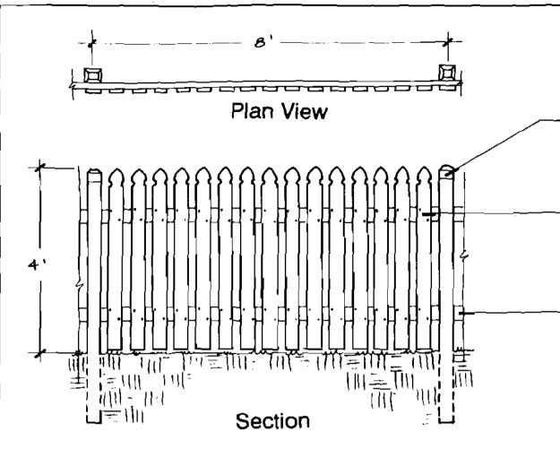
Posts are made of Oak or pressure treated wood and are 4"x4" x7'.
