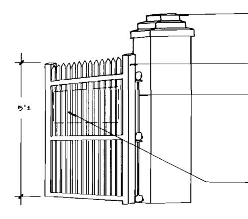
Column is approximately  $16" \times 16" \times 6'$ . Column can be constructed of brick and left natural or painted dark brown or medium brown to match proposed fence.
