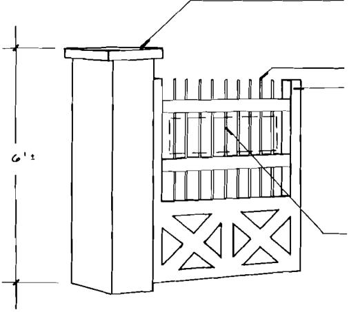
Column is approximately 16" x 16" x 6. Column can be constructed of brick and left natural or painted dark brown or gray to match proposed fence.
