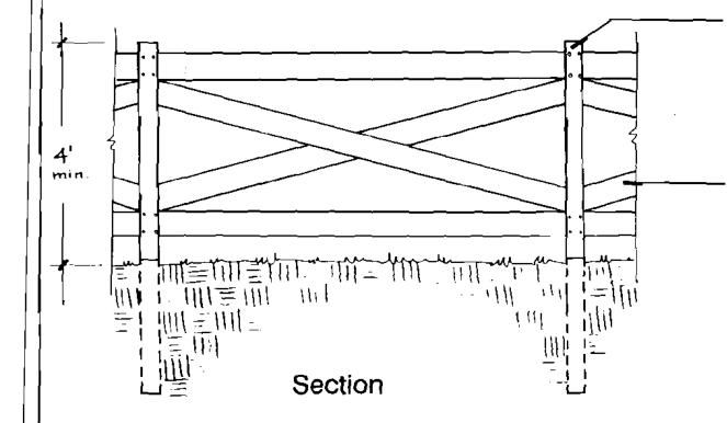
Posts are made of hardwood and are 3" × 6" × 7". Posts are set approximately 33" into the ground. Posts are to be faced with hardwood or pressure treated wood to match fence boards. Posts should be pressure treated to protect from rotting.
