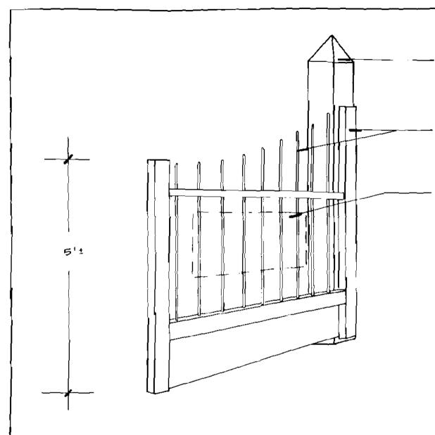
Pencil post is made of wood and is approximately 6" × 6" × 8". Wood post can be pressure treated or Oak. Wood can be natural, stained or painted dark brown.
